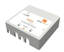
The dSCR GTU converts optical power to RF power (4 satellite bands and FM,DAB,DTT). Terrestrial signals are overlaid onto both output ports. All units have built in AGC which allows a wide dynamic range of optical levels without affecting output power and quality. One LED indicator allows the user to monitor the status of the unit. Able to work in legacy, analogue SCR (aSCR) and digital SCR (dSCR) modes.
